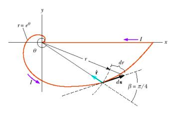
To complete a loop, the ends of the spiral are connected by a straight wire along the *x* axis. Find the magnitude and direction of  $\vec{B}$  at the origin.
