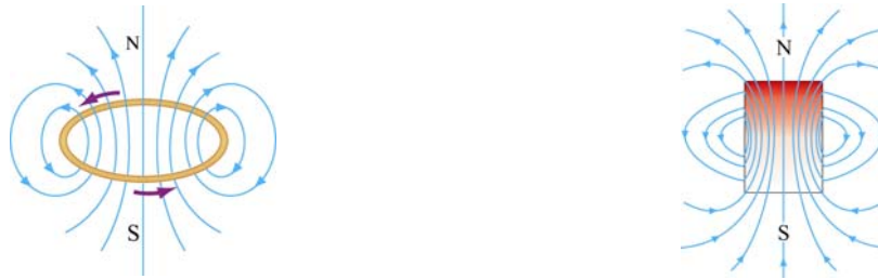
Figure 9.8.3 Magnetic field lines due to (a) a current loop, and (b) a small bar magnet.
