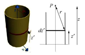
We locate the area element at the point  $(R, \varphi', z')$ . Note that  $(\varphi', z')$  are the integration variables. (Note that is the reason we prime these coordinates.) A small area element is given by
