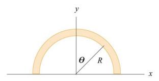
The total charge on the semicircle is Q. However, the charge per unit length along the semicircle is non-uniform and given by  $\lambda = \lambda_0 \cos \theta$ .
