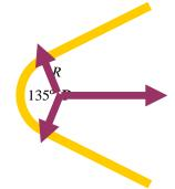
Drawing our three E field vectors, it is clear that the vertical components of from the lines will cancel as well, so we only need the horizontal component. I'll figure it out for the bottom line and double it. Since the line is rotated down by 22.5° (half of the 45° between the lines), the E field angle is rotated from 45° to 67.5°. We want the horizontal component of that:
