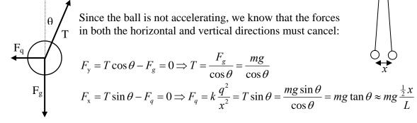
where we have used the small angle approximation that  $\tan \theta \approx \sin \theta$ , which is valid when the length of the string L is long (relative to the separation x), which we are told it is. Continuing:
