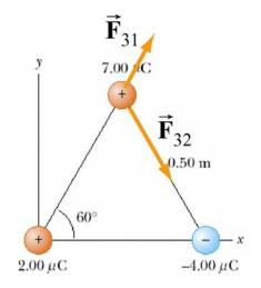
$$F_{31} = \frac{1}{4\pi\varepsilon_0} \frac{q_3 q_1}{r^2} = \frac{\left(8.99 \times 10^9 \text{ N} \cdot \text{m}^2/\text{C}^2\right) \left(7.00 \times 10^{-6} \text{ C}\right) \left(2.00 \times 10^{-6} \text{ C}\right)}{\left(0.500 \text{ m}\right)^2} = 0.503 \text{ N}$$
