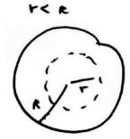
The sphere has a uniform charge density  $\rho = Q/(4/3)\pi R^3$ . Because the charge distribution is uniform, the charge enclosed in our Gaussian surface is given by
