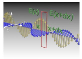
b) Use Faraday's Law (with the rectangular loop pictured at left) to calculate a relationship between the spatial derivative of the electric field and the time derivative of the magnetic field.
