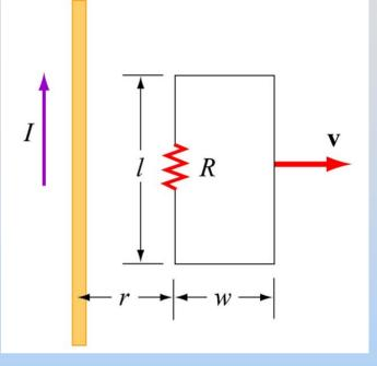
**Note**:  $I_{ind} dI \ge B$  force is left on the left segment and right on the right, but the force on the left is bigger. So the net force on the rectangular circuit is to the left, again trying to keep the flux from decreasing by slowing the circuit's motion
