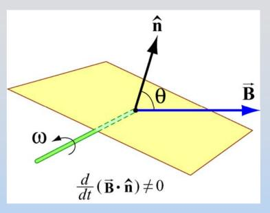
**Note**:  $I_{ind} dI \ge B$  force on the sides of the square loop will be such as to produce a torque that tries to stop it from rotating (Lenz's Law).
