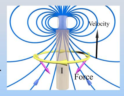
The I dI x B force on the coil is a force which is trying to keep the flux through the coil from increasing by slowing it down (Lenz's Law again).
