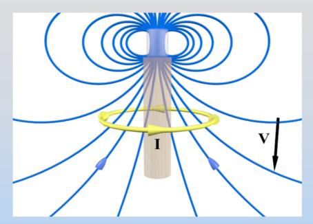
A conducting loop is below a magnet and moving downwards. This induces a current as pictured. The *I* ds x B force on the coil is
