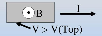
Look at the force on the carriers. If positive, they are flowing to the right, and **F** will be down. If negative they are flowing to the left and **F** will be down (don't forget the sign of q!) So either way the force is down. But we know that the result is a higher potential at the bottom – positive charges are moving down. So the carriers are positive
