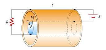
conductors at the other end of the cable. A current I flows down the inner conductor and back up the outer one. The battery charges the inner conductor to a charge -Q and the outer conductor to a charge +Q.
