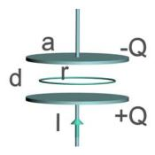
Choose for an Amperian loop, a circle of radius r < a in the plane midway between the plates. Calculate the line integral of the magnetic field around the circle,  $\int_{-\mathbf{B}}^{\mathbf{I}} \mathbf{B} \cdot d\mathbf{s}$ .
