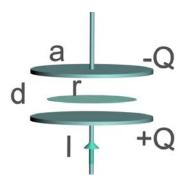
Using your expression for  $\vec{\mathbf{E}}$  above, calculate the electric flux through this flat disk of radius r < a in the plane midway between the plates, in terms of r, Q(t), a, and  $\varepsilon_0$ . Take the surface normal to the imaginary disk to be in the  $\hat{\mathbf{k}}$  direction.
