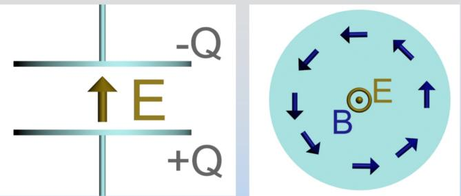
The figures above show a side and top view of a capacitor with charge *Q* and electric and magnetic fields E and B at time *t*. At this time the charge *Q* is:
