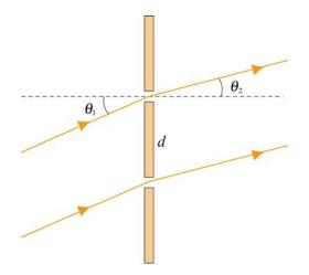
If an interference maximum is formed at an angle  $\theta_2$  far from the slits, find the relationship between  $\theta_1$ ,  $\theta_2$ , d and  $\lambda$ .
