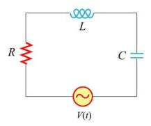
Consider the circuit at left, consisting of an AC function generator ( $V(t) = V_0 \sin(\omega t)$ , with  $V_0 = 5$  V), an inductor L = 8.5 mH, resistor R = 5  $\Omega$ , capacitor C = 100  $\mu$ F and switch S.
