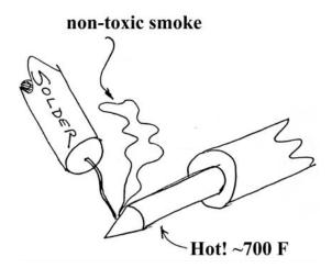
**Figure 1: Tinning the soldering iron**
