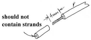
**Figure 3: Stripping wires**
