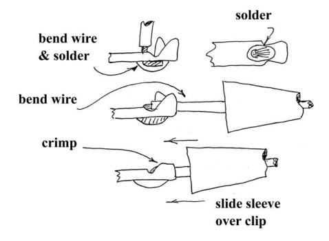
**Figure 5: Soldering clip leads**
