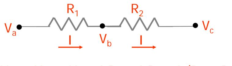
$$V_{ac} = V_{ab} + V_{ac} = I R_1 + I R_2 = I (R_1 + R_2)$$
