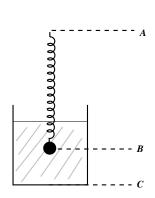
The cup is now moved up and down at an angular frequency  $\omega$ . The position of the bottom of the cup (C) is given by  $d_1(t) = D_1 \cos(\omega t)$ .
