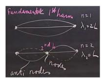
(16:30). By driving at appropriate frequencies, the resonances corresponding to the normal modes can be easily excited, as has been demonstrated many times, and is done here for the modes on stretched strings.
