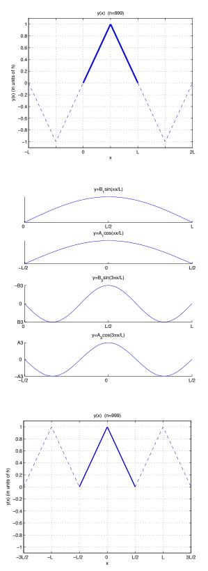
Since this Fourier decomposition gives the shape of the original function in the interval [-L/2, L/2], it is a correct mathematical solution. In part (c), however, we will see that this decomposition is not physically correct if we let the string evolve in time.
