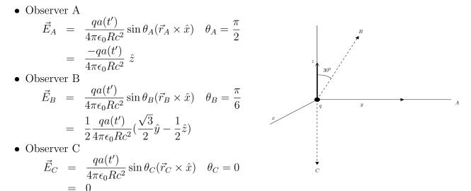
**b)** As |B| = |E|/c, hence the relative strengths of the magnetic field *B* are the same as the relative strengths of the electric field *E* in Part(a) at the three observation points. The arrival time of the magnetic field at the three observers *A*, *B* and *C* is  $t_{arrival} = R/c$ . The direction of the induced magnetic field at the three points is in the  $-\hat{x}$  direction.
