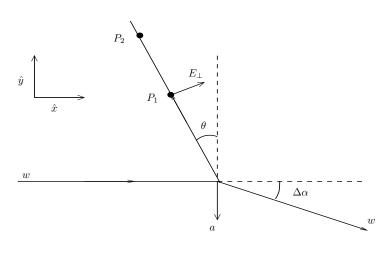
where  $a_{\perp}$  is the component of acceleration perpendicular to the position vector of the distant point  $P_1$ . Then the electric field at point  $P_1$  is anti-parallel to  $a_{\perp}$  and is oriented as shown in the figure.
