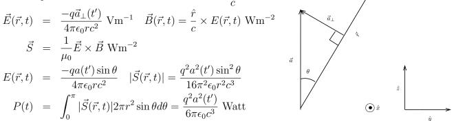
a) Arrival time at all the three observers A, B and C is  $t_{arrival} = R/c$ . The direction of the electric field at the point of observation is anti-parallel to the component of the acceleration perpendicular to the position vector. The direction of the magnetic field is the cross product of the position vector with the electric field. The figure below shows the directions to the 3 observers.
