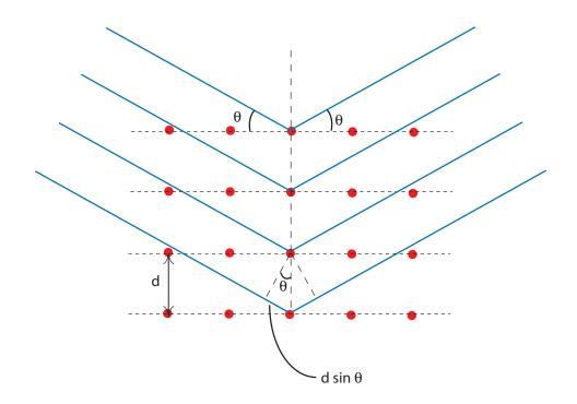
The Davisson and Germer experiment is different in that the incoming beams of electron waves are at normal incidence (see diagram). Thus, we need a modified Bragg relation for this new geometry. If we imagine the electrons scattering off the surface layer of atoms, constructive interference occurs when (as usual) the path difference is an integer multiple of the wavelength:
