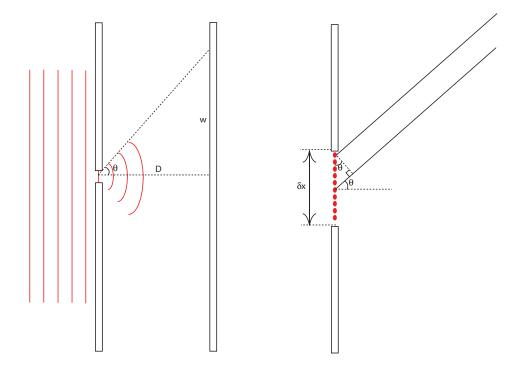
(b) (5 points) The photons with the greatest transverse momentum will be those at the edge of the pattern. For such photons, their travel direction is given by  $\theta = \frac{\delta p_x}{p}$ , which combines with  $\theta \approx w/D$  to give
