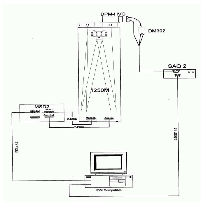
FIG. 2: Schematic of the Jobin Yvon 1250M monochromator.
