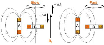
FIG. 2: Semiclassical explanation for spin-spin coupling, showing two spins in a strong magnetic field  $B_0$ . Each spin produces its own local magnetic field, which is seen by its neighbor. When spin A is spin-up, its field subtracts from that seen by B, thus causing it to precess slower. When A is spin-down, its field adds, causing B to precess faster. A is a quantum spin which only has two states.
