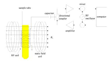
FIG. 6: Schematic diagram of an NMR apparatus.
