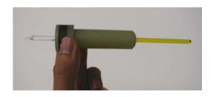
FIG. 5: Picture of a typical NMR sample in a spinner.
