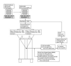
FIG. 4: An overview of the Bruker acquisition system.
