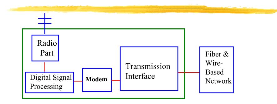
WSB architectures are -integral & proprietary Suppliers include: Nortel, Moto, Ericsson, Siemens, Nokia Disruptive Modem advances (e.g., MUD) can double Base Station Capacity
