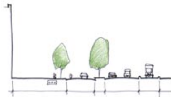
figure 3: street Adaptability: Streets should be designed to adapt to future needs. Above, a median designed for the short term can become a rapid transit right-of-way in the long term.
