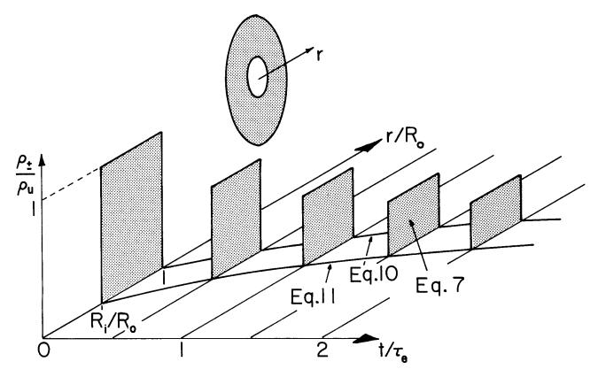
Fig. 5.6.3. When t = 0, a uniform density  $\rho_u$  of charged particles fills the spherical shell  $R_i \le r \le R_o$ . A source of gas at the origin imparts a radial velocity. For this plot,  $R_o/R_i$  = 0.5,  $3\Phi_v\tau_e/4\pi R_o^3$  = 1. Remember that the charge is self-precipitating in three dimensions. At any time, the product of the charge density and the volume of the region filled by the charge is constant.
