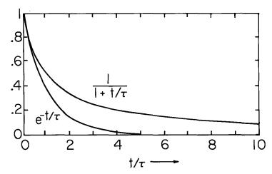
Fig. 5.6.2. Comparison of self-presipitation transient to exponential decay.
