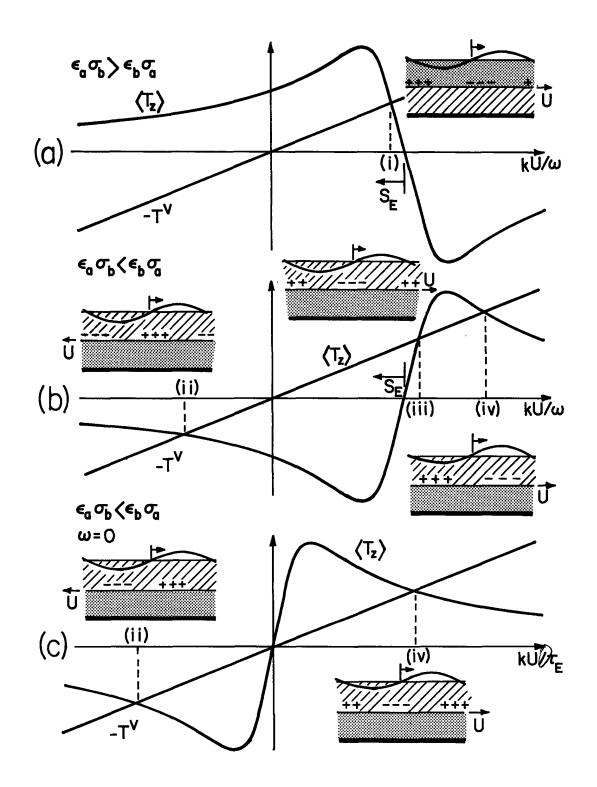
Fig. 5.14.3. Dependence of electric space-average surface force density on material velocity.
