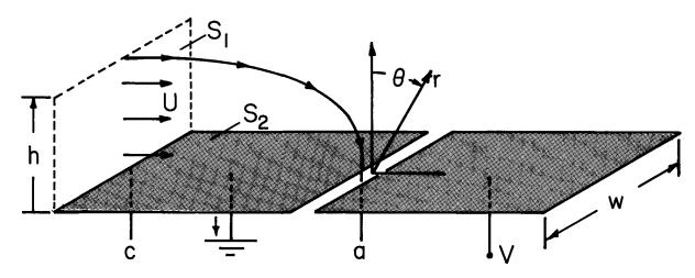
Fig. 5.4.1. Electrodes embedded in a smooth wall have the potential difference V.
