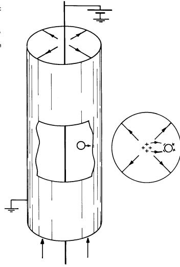
Fig. 5.5.1. Single-stage tube-type electrostatic precipitator.
