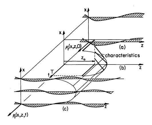
Fig. 5.10.1. (a) The initial distribution of charge density as a function of (x,z). (b) Characteristic lines in (x,z,t) space. Those lines originating along the cross section  $z=z_0$  when t=0 are shown. (c) Distribution of charge density by the time t=T. Charge is transported downstream in proportion to the stream velocity, and decays as  $\exp(-t/\tau_0)$ .
