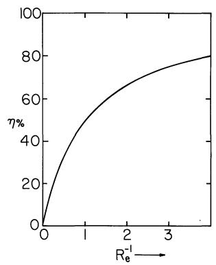
Fig. 5.6.5. Efficiency of space-charge precipitator as function of reciprocal electric Reynolds number, the ratio of residence time to t<sub>s</sub>.
