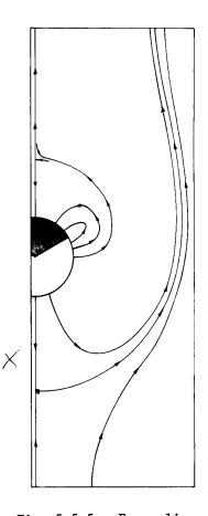
Fig. 5.5.5. Force lines in detail for regimes (e) for positive ions and (h) for negative ions. Here, all of the characteristic lines terminating on the particle also originate on the particle; hence, there is no charging. For the case shown, U = +2bE, q = +q<sub>C</sub>/2.
