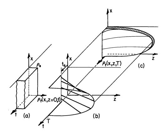
Fig. 5.10.2. (a) When t = 0, a uniform and henceforth constant source of charge is turned on at z = 0. (b) Characteristic lines. (c) Later distribution of charge density.
