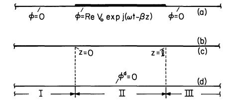
Fig. 5.17.3. A thin sheet moving with velocity U in the z direction enters the excitation region at z = 0 and leaves at  $z = \ell$ .
