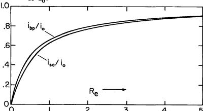
Fig. 5.7.4. Dependence of the normalized short-circuit and zero-pressure-drop currents on n the electric Reynolds number  $R_{\rm e}$ .
