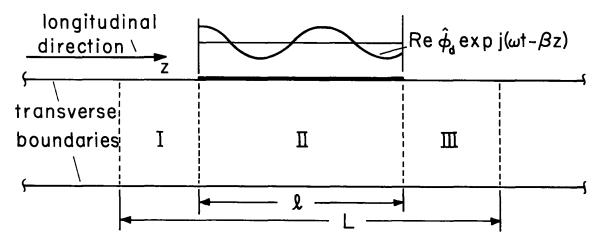
Fig. 5.17.1. Abstract view of systems having excitation on transverse boundaries which are in the temporal sinusoidal steady state but confined to the region \( \ell. \).
