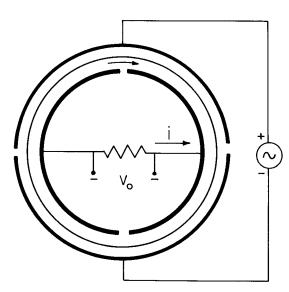
Fig. 5.13.4. Adaptation of the planar configuration of Fig. 5.13.3 to measure rotational velocity of shell of slightly conducting material.
