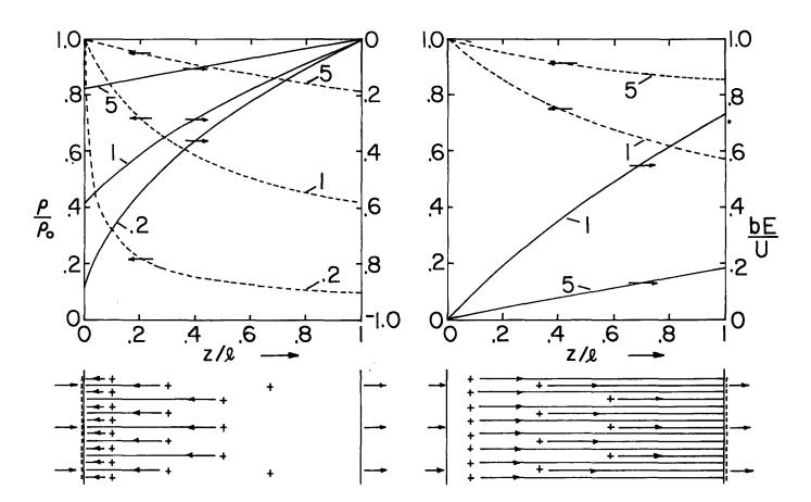
Fig. 5.7.7. Distribution of charge density and electric field intensity for generator and pump. The parameter  $R_{e}\equiv(\epsilon/b\rho_{o})/(\hbar/U)$  can be regarded as a normalized velocity.
