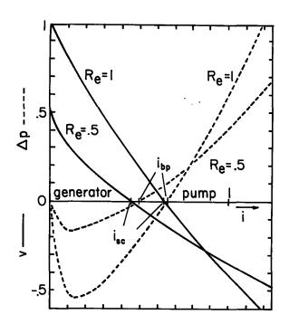
Fig. 5.7.3. Electrical and mechanical terminal characteristics as a function of the normalized terminal current with the electric Reynolds number  $R_e$  as a parameter. v is normalized to  $\rho_0 \ell^2/\epsilon,~\Delta p$  is normalized to  $(\rho_0 \ell)^2/2\epsilon,~and~i$  to  $i_0.$
