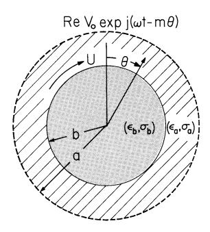
Fig. 5.14.1. Cross-sectional view of two planar layers of material having thicknesses a and b, respectively. The potential is constrained to be a traveling wave just above, and to be constant just below.
