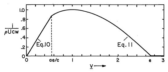
Fig. 5.4.3. Normalized current to electrode in Fig. 5.4.1 as function of normalized voltage  $V = bV/\pi Uc$ .
