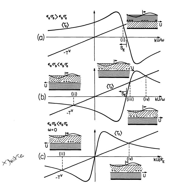
Fig. 5.14.3. Dependence of electric space-average surface force density on material velocity.
