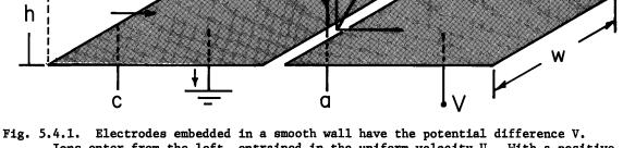
Fig. 5.4.1. Electrodes embedded in a smooth wall have the potential difference V. Ions enter from the left, entrained in the uniform velocity U. With a positive V, the left electrode intercepts some of the ions from the flow.
