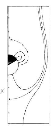
Fig. 5.5.5. Force lines in detail for regimes (e) for positive ions and (h) for negative ions. Here, all of the characteristic lines terminating on the particle also originate on the particle; hence, there is no charging. For the case shown,  $U = \pm 2bE$ ,  $q = \pm q_c/2$ .
