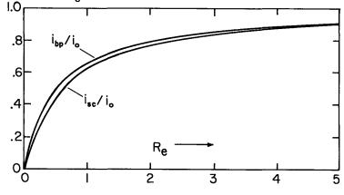
Fig. 5.7.4. Dependence of the normalized shortcircuit and zero-pressure-drop currents on n the electric Reynolds number Re.
