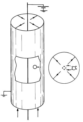
Fig. 5.5.1. Single-stage tube-type electrostatic precipitator.
