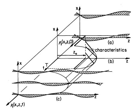
Fig. 5.10.1. (a) The initial distribution of charge density as a function of (x,z). (b) Characteristic lines in (x,z,t) space. Those lines originating along the cross section  $z = z_0$  when t = 0 are shown. (c) Distribution of charge density by the time t = T. Charge is transported downstream in proportion to the stream velocity, and decays as  $exp(-t/\tau_o)$ .
