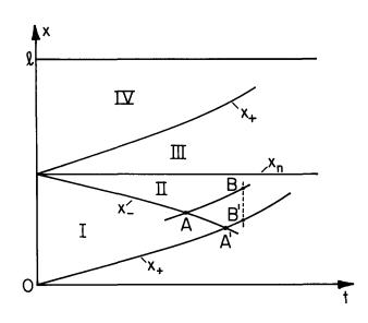
Fig. 5.9.4. Regions in x-t plane delimited by characteristic lines emanating from initial interface position.
