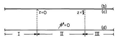
Fig. 5.17.3. A thin sheet moving with velocity U in the z direction enters the excitation region at z = 0 and leaves at  $z = \ell$ .
