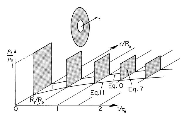
Fig. 5.6.3. When t = 0, a uniform density  $\rho_u$  of charged particles fills the spherical shell  $R_i < r < R_o$ . A source of gas at the origin imparts a radial velocity. For this plot,  $R_o/R_i = 0.5$ ,  $3\Phi_v \tau_e/4\pi R_o^3 = 1$ . Remember that the charge is self-precipitating in three dimensions. At any time, the product of the charge density and the volume of the region filled by the charge is constant.
