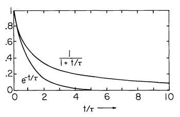
Fig. 5.6.2. Comparison of self-presipitation transient to exponential decay.
