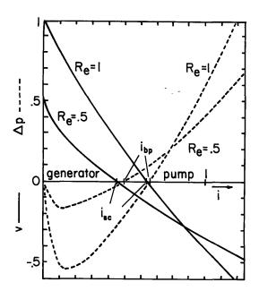
Fig. 5.7.3. Electrical and mechanical terminal characteristics as a function of the normalized terminal current with the electric Reynolds number Re as a parameter. v is normalized to  $\rho_0 l^2/\epsilon$ ,  $\Delta p$  is normalized to  $(\rho_0 l)^2/2\epsilon$ , and i to io.
