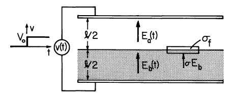
Fig. 5.9.2. Maxwell capacitor model for bipolar migration of Fig. 5.8.6.
