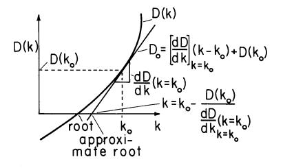
Fig. 5.17.5. Numerical solution illustrated graphically. The zero of the complex function D(k) of the complex variable is approximated at the trial value  $k_0$  by a straight line. The approximate root follows by setting  $D_0(k) = 0$ . This root can then be used as  $k_0$  in refining the approximation and the process repeated until the desired accuracy is obtained. To obtain roots of Fig. 5.17.6,  $k_0$  is first approximated by Eqs. 11 and 13.
