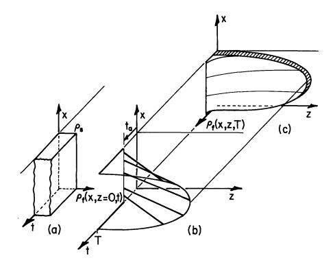
Fig. 5.10.2. (a) When t = 0, a uniform and henceforth constant source of charge is turned on at z = 0. (b) Characteristic lines. (c) Later distribution of charge density.
