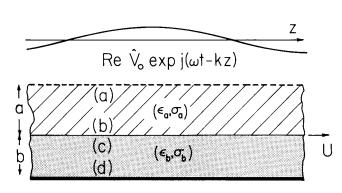
Fig. 5.14.1. Cross-sectional view of two planar layers of material having thicknesses a and b, respectively. The potential is constrained to be a traveling wave just above, and to be constant just below.
