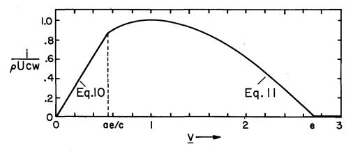
Fig. 5.4.3. Normalized current to electrode in Fig. 5.4.1 as function of normalized voltage  $\underline{V} = b\nabla/\pi Uc$ .
