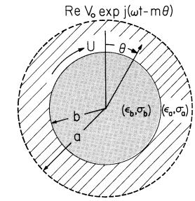
tem of Fig. 5.14.1. Qualitatively, fields in the planar problem are the same as those in this circular configuration if the z axis of Fig. 5.14.1 is wrapped around on itself in an integral number of wavelengths.
