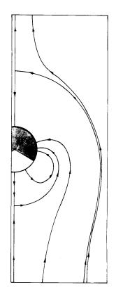
Fig. 5.5.6. Regimes (h) for positive ions and (e) for negative ions. Some of the characteristic lines extend to where the charge enters.  $U = \pm 2b \pm E$ ,  $q = \pm q_c/2$ .
