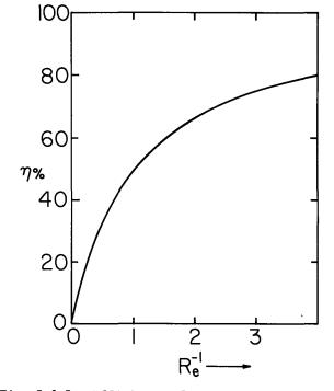
Fig. 5.6.5. Efficiency of space-charge precipitator as function of reciprocal electric Reynolds number, the ratio of residence time to  $\tau_e$ .
