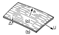
Fig. 6.3.1. Conducting sheet having normal flux density  $B_n$ , thickness  $\Delta$  and hence surface conductivity  $\sigma_8$  =  $\Delta\sigma_*$
