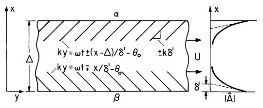
Fig. 6.8.1. Lines of constant phase move to right with velocity  $\omega/k$ . For  $\omega/k$  exceeding U, these lines form a "wake" to the left, as shown. If material velocity were to exceed  $\omega/k$ , lines would slant to the right. Amplitude decays into material as shown, with depth for attenuation by  $e^{-1}$  equal to  $\delta'$ .
