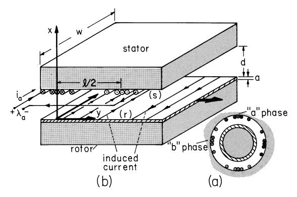
Fig. 6.4.1. (a) Cross section of rotating induction machine with thin-sheet conductor on rotor. (b) Developed model for (a) with air gap d and sheet conductor of thickness a. One of two phases on the stator is shown.
