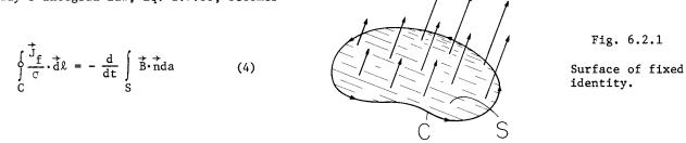
In writing this equation, the surface S enclosed by the contour C, Fig. 6.2.1, is one of fixed identity (one attached to the deforming material), so  $\vec{v} = \vec{v}_s$ . (The same expression would be obtained by integrating Eq. 3 over a surface of fixed identity and applying the generalized Leibnitz rule, Eq. 2.6.4.)
