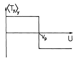
Fig. 6.11.4. Dependence of magnetic surface force density on speed for a hysteresis-type device.
