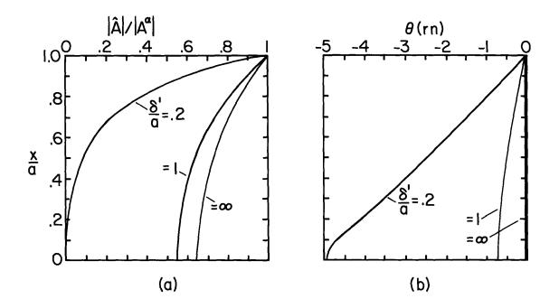
Fig. 6.6.3. Amplitude and phase of  $A = Re|\hat{A}(x)|exp j(\omega t - ky + \theta(x)|$  for fields diffusing through conductors of Fig. 6.6.1. The parameter is the skin depth, based on the material frame frequency, normalized to the conductor thickness,  $\delta'/a$ ; ka = 1.
