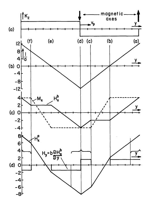
Fig. 6.4.3. (a) Distribution of surface current on "stator." (b) I/a; (c) distribution of magnetization and perpendicular magnetic field intensity in moving member; and (d) field components in adjacent air gap.
