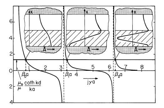
Fig. 6.10.2. Graphical solution for eigenvalues  $(j\gamma_n a)$  satisfying Eq. 6. Inserts show associated eigenfunctions,  $\hat{A}(x)$ , with ka = kd = 1 and  $\mu/\mu_0$  = 1. Roots shown are  $\beta_0 a = 0.776$ ,  $\beta_1 a = 3.364$  and  $\beta_2 a = 6.401$ .
