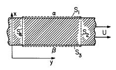
Fig. 6.7.1. Control volume fixed in laboratory frame with fundamental periodicity length in y direction.
