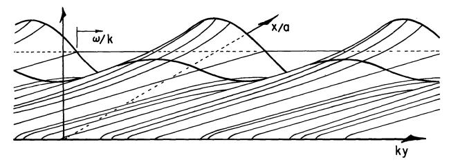
Fig. 6.6.4. Magnetic diffusion wave distribution A across conducting layer of Fig. 6.6.1 with pure traveling wave of excitation. For fields shown, phase velocity  $\omega/k$  of wave exceeds material velocity U. As time proceeds, picture translates to the right with phase velocity  $\omega/k$ .
