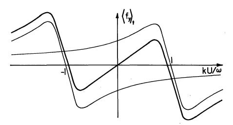
Fig. 6.4.4. Time-average force for single-phase induction machine as function of material velocity normalized to wave velocity. Total force is superposition of forces due to forward and backward wave components.
