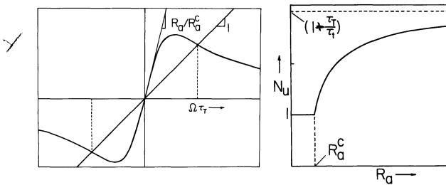
Fig. 10.5.4. Vertical heat flux normalized to flux in absence of rotation as a function of  $R_a$ .
