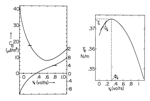
Fig. 10.11.2a. Incremental capacitance and charge per unit area as function of voltage for mercury-KNO<sub>3</sub>. Here the electrolyte is 0.2 M KNO<sub>3</sub> in gel. This solid-liquid interface exhibits properties typical of liquid-liquid interfaces.<sup>3</sup>
