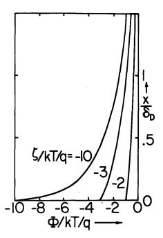
Fig. 10.8.1. Potential distribution in diffuse part of double layer with zeta potential as parameter.
