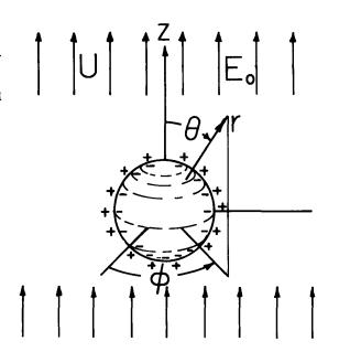
Fig. 10.10.1. Solid insulating particle supporting double layer.
