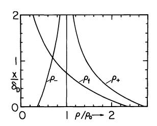
Fig. 10.8.2. Charge density distributions for  $\zeta = kT/q$ .
