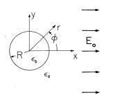
**Fig. 6.6.5** Insulating rod having uniform permittivity  $\epsilon_b$  surrounded by material of uniform permittivity  $\epsilon_a$ . Uniform electric field is imposed by electrodes that are at "infinity."
