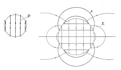
Fig. 6.3.1 Equipotentials and lines of electric field intensity of permanently polarized sphere having uniform polarization density. Inset shows polarization density and associated surface polarization charge density.
