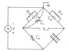
Fig. 6.6.4 Balanced amplifiers of oscilloscope, balancing capacitors, and demonstration capacitor shown in Fig. 6.6.4 comprise the elements in the bridge circuit. The driving voltage comes from the transformer, while  $v_o$  is the oscilloscope voltage.
