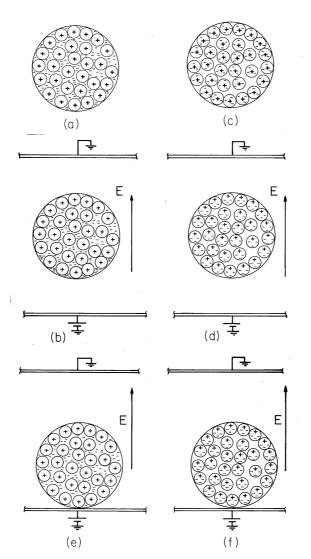
Fig. 6.0.1 In the left-hand sequence, the sphere is conducting, while on the right, it is polarizable and not conducting.
