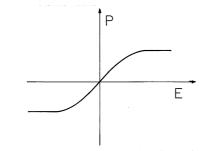
Fig. 6.4.1 Polarization characteristic for nonlinear isotropic material.
