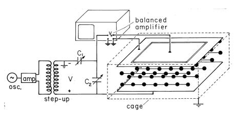
Fig. 6.6.3 Demonstration in which change in capacitance is used to measure the equivalent dielectric constant of an artificial dielectric.
