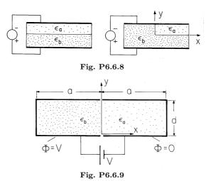
between the plane parallel electrodes of Fig. P6.6.8. In Fig. P6.6.8a, there are two layers of dielectric.
