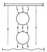
Fig. 6.6.2 From the microscopic point of view, the increase in capacitance results because the dipoles adjacent to the electrode induce image charges on the electrode in addition to those from the unpaired charges on the opposite electrode.
