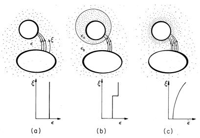
Fig. 6.5.1 Field region filled by (a) uniform dielectric, (b) piece-wise uniform dielectric and (c) smoothly varying dielectric.
