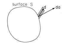
Fig. 6.1.1 Volume element containing positive charges which have left negative charges on the other side of surface S.
