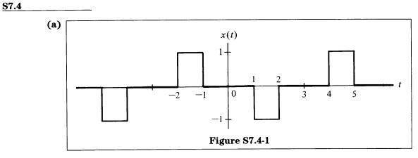
Note that the period is  $T_0 = 6$ . Fourier coefficients are given by
