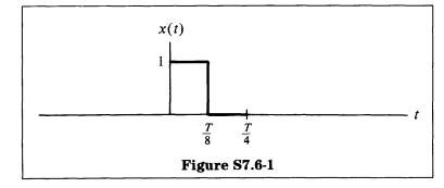
(a) Since x(t) is even, we can extend Figure S7.6-1 as indicated in Figure S7.6-2.
