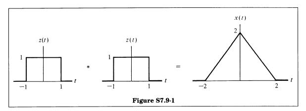
(b) Since z(t) \* z(t) = x(t), as shown in Figure S7.9-1, then  $\tilde{z}(t)$  is shown in Figure S7.9-2.
