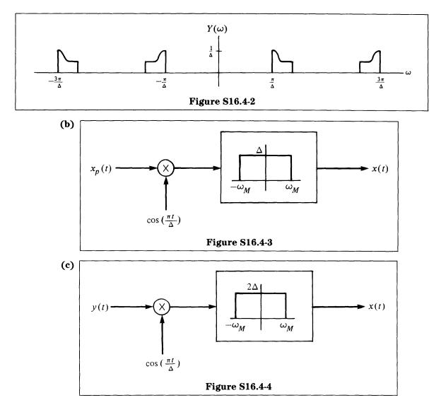
(d)  $\Delta$  is maximum when  $\pi/\Delta$  is minimum. From part (a) we see that aliasing is avoided in  $X_p(\omega)$  if  $\omega_M \leq \pi/\Delta$ . Hence,  $\Delta_{\max} = \pi/\omega_M$ .
