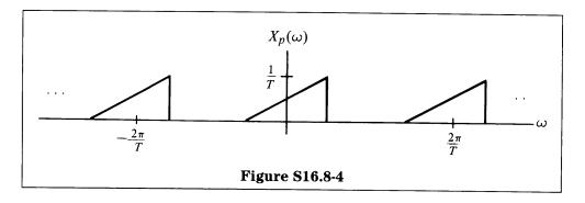
**(b)**  $2\pi/T_{\text{max}}$  equals the Nyquist rate for  $X_2(\omega)$ :
