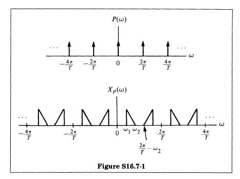
Note that as T increases,  $(2\pi/T) - \omega_2$  approaches  $\omega = 0$ . Also, there is aliasing when  $2\omega_1 - \omega_2 < (2\pi/T) - \omega_2 < \omega_2$ . If  $2\omega_1 - \omega_2 \ge 0$  (as given in the problem), then it is easy to see that there is no aliasing when  $0 \le (2\pi/T) - \omega_2 \le 2\omega_1 - \omega_2$ . For maximum T, we choose a minimum allowable value of  $2\pi/T$ :
