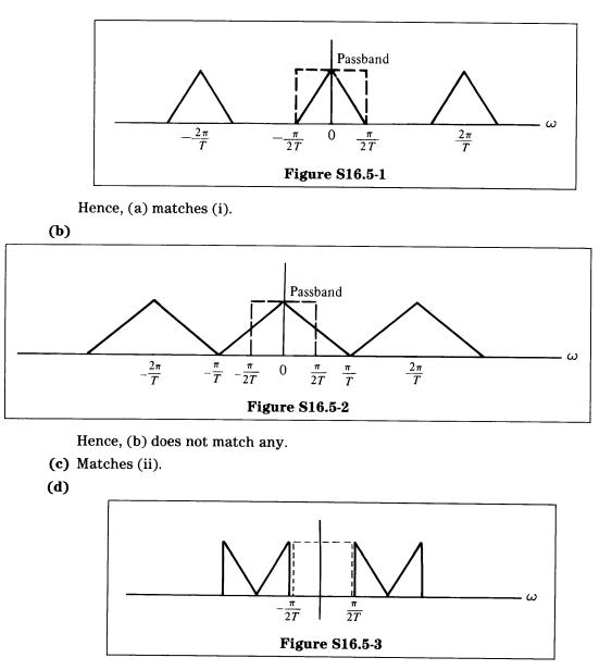
(a) The transform of the sampled function appears as in Figure S16.5-1.
