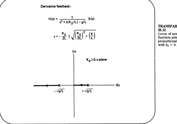
TRANSPARENCY 26.12 Locus of system function poles for proportional feedback TRANSPARENCY 26.13 Overall system function with proportional plus derivative feedback.
