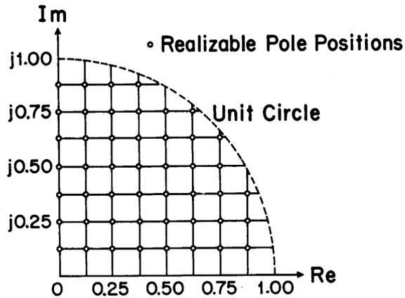
Grid of possible pole locations for the network of viewgraph d when the coefficients are quantized to three bits.
