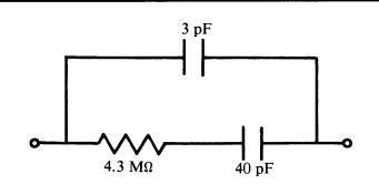
Figure S13.3 Modified compensation network for Problem 13.2 (P13.11).
